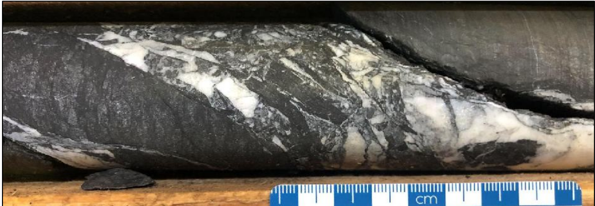
Figure 16: Minor Fault at 76.4m
