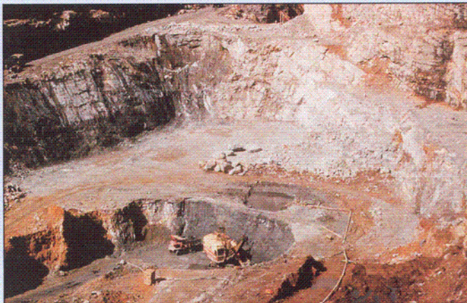
Mining the last of the secondary (oxide) ore at the Tynagh Pb-Zn-Cu-Ag open-pit.
