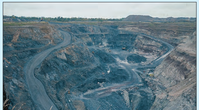
Gortdrum Cu-Ag-Hg open-pit, looking E. Devonian sandstones on right (brown) thrust over Lower Carboniferous limestones on left (grey).
